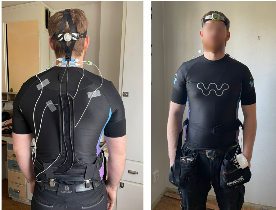
Figure 5 Full set-up of EMG and IMU equipment while wearing Spineband
