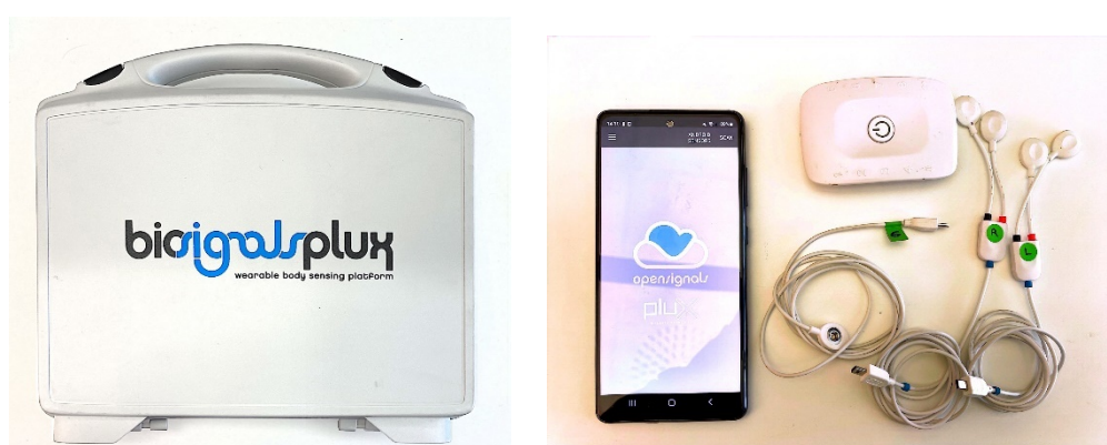
Figure 4 EMG equipment from Biosignalsplux' Researcher kit, consisting of a phone application, three cables and a logger
