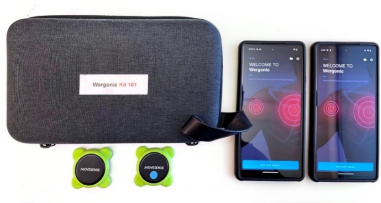
Figure 3 Wergonic Kit consisting of two IMU sensors and a phone application to measure postural data
