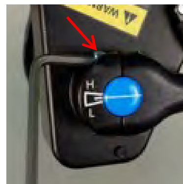
Figure 17: Loosening End Link Screw
