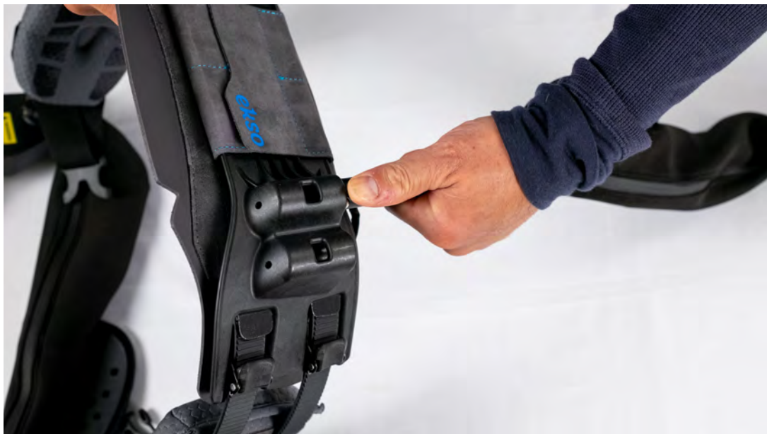
Figure 10: Installing Ekso EVO Arms
