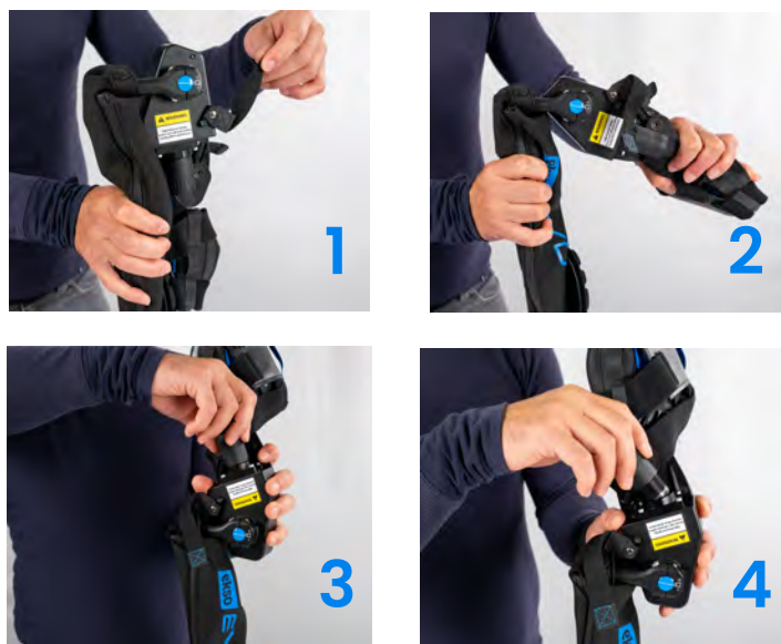
Figure 15: Installing Actuator Springs
